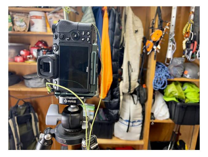
It allows vertical shots to be centered over the tripod, instead of out to the side.
